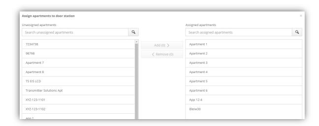
Picture 8.7: Assigning apartments to the door station
